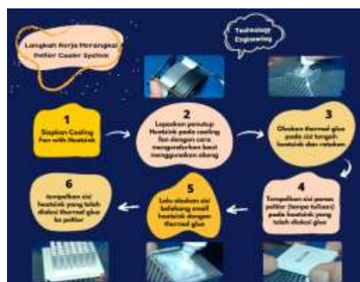
Figure 5. Steps to assemble the system cooler peltier
